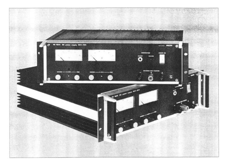
These 400W and 1000W power supplies use the thyristor, pre-regulation technique and a unique design feature that increases efficiency and reliability whilst reducing cost. They are ideal for both laboratory and OEM applications, having comprehensive systems facilities. Separate volt and ammeters, coarse and fine potentiometers, bright LED displays for mode indication and automatic indication of crossover also make the units simple and convenient to use.
